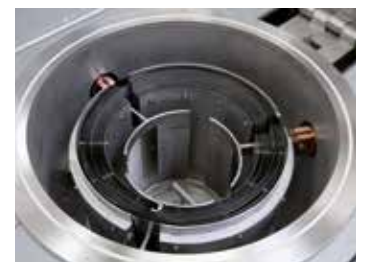
Cylindrical retort with tungsten heating
