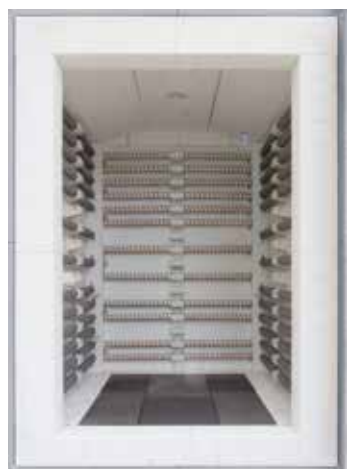
Chamber furnace N 650/14 BO with ignition burner
