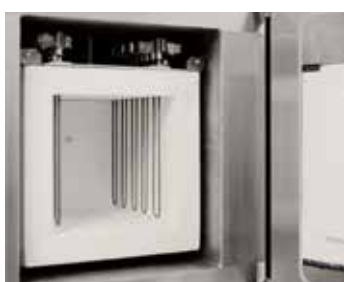
Molybdenumdisilicide heater and fiber insulation
