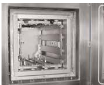
Molybdenum or tungsten heating chamber
