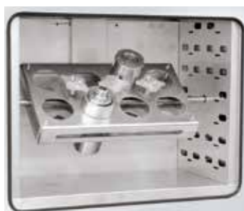
Electrical rotating device as additional equipment
