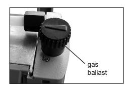
For **condensable vapors** (water vapor, solvents, etc.):
