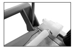
► Loosen the screw affixing the handle (use 5 mm wide Allen key) at one housing cover.
