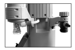
Remove catchpots (10) at inlet and outlet (see "Use and operation", pg. 38).
