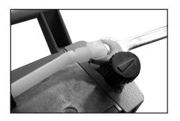
Slip the hose onto the hose connector by turning the fitting (L) with an open-ended wrench w/f 14
