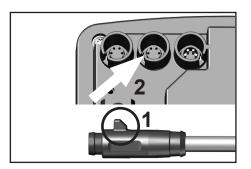
Depending on technical version the connections of the VACUU•BUS cables are equipped with a nib.
