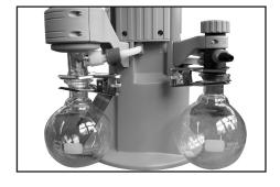
→ Assemble catchpots (10) with joint clips.
