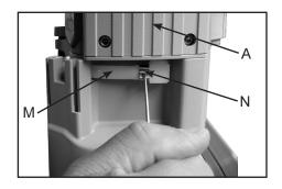
Detach the coupling of the hose connection (M) below the housing cover (A).
