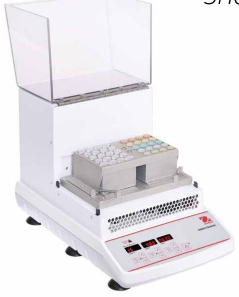
OHAUS Incubating Cooling Orbital Shakers are designed to incubate samples from 10°C below ambient to 65°C. Incubating Cooling Mini Shaker is designed to hold two microplates or two optional modular tube blocks in a variety of configurations. All models feature touchpad controls with easy-to-read, independent LED displays for temperature, speed and time. Microprocessor control provides consistent uniform shaking action.
