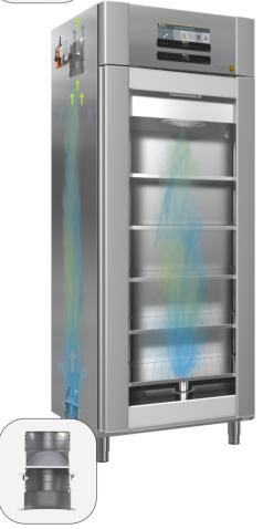
Ambient air is drawn into the cabinet interior through a check valve when the damper opens, equalising the pressure in the interior thereby flushing out potentially contaminated air.
