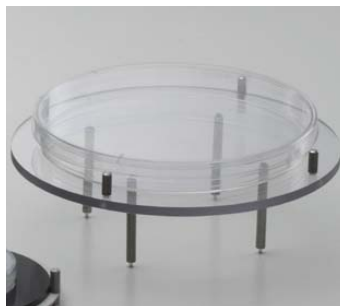
Adapter for Petri dishes with Ø 140-150 mm
