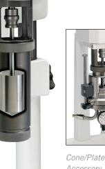
Cone/Plate Accessory provides extended range capability for shear rate and viscosity
