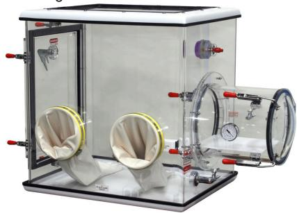
The 810-SG Series by PLAS—LABS are constructed of an optically clear material, developed for isolation and / or containment. All units feature a high visibility of the interior, cleanliness, safety, complete containment, portability and a draft-free atmosphere. The installed purging valves are ideal for lowering oxygen and humidity levels.
