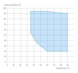
Note: Within the respective temperature-humidity range, permanent operation is possible (at an ambient temperature of 22 °C  $\pm$  3 K; relative humidity < 50 %). Condensation may occur in the threshold range. To which extent depends on the humidity content of the chamber load and the ambient conditions.
