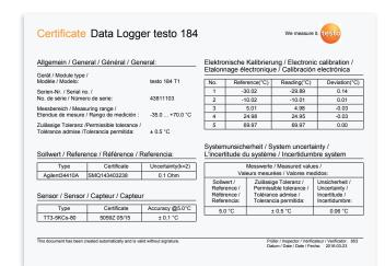
Temperature data loggers testo 184 T1, T2, T3, and T4 come with an acceptance test certificate according to DIN ISO 10204. Further traceable calibration certificates according to ISO 17025 or DAkkS are available on request.
