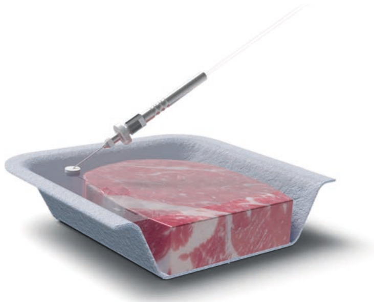
Taking a protective gas mixture sample from a food package
