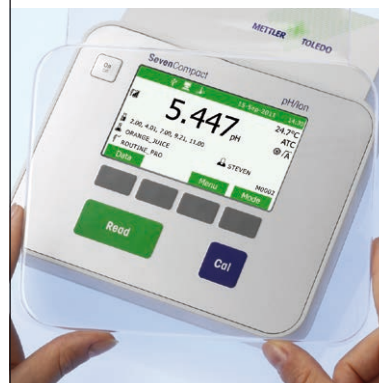
Transparent cover as an extra barrier
